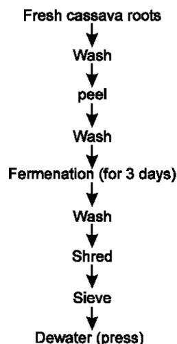
Fig. 1: Flow chart of cassava processing into fermented pulp
