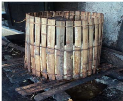
Fig. 6: Gambir paste surrounded by bamboo to reduce the water content
