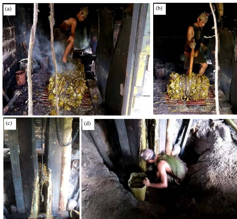
Fig. 4 (a-d): (a) A farmer arranging Uncaria gambir leaves and branches after steaming, (b) Cylinder form of Uncaria gambir leaves and branches ready for pressing, © Pressing process using mechanical extraction and (d) Collection of the extract
