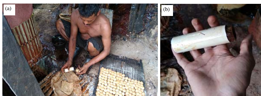
Fig. 7(a-b): (a) A farmer forms the gambir paste and (b) Die used to form gambir
