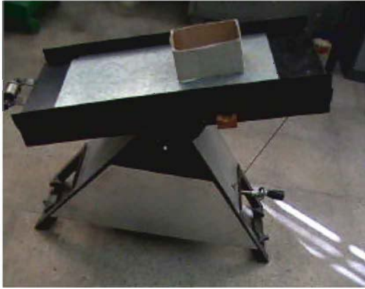
Fig. 1: Apparatus for measuring static coefficient of friction.
