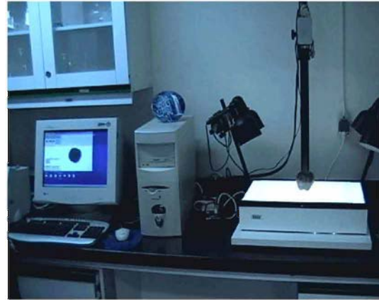
Fig. 2: Area Measurement System-Delta Tenglend for measuring projected area of apples.
